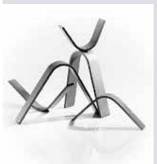
MARS® 600 thickness 8.7 mm
